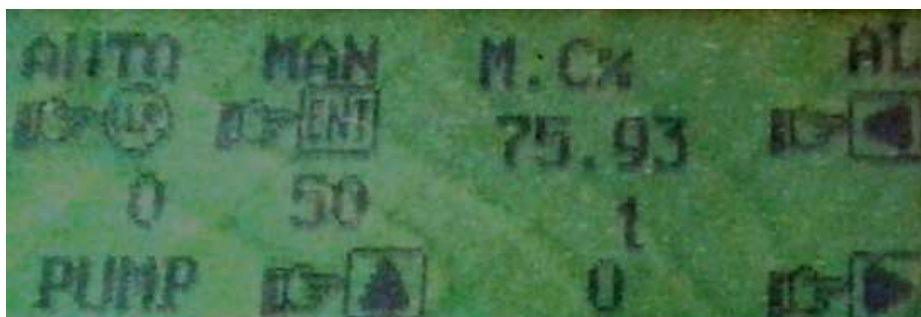
Figure 4. Moisture content value and operation data shown on the digital screen.
